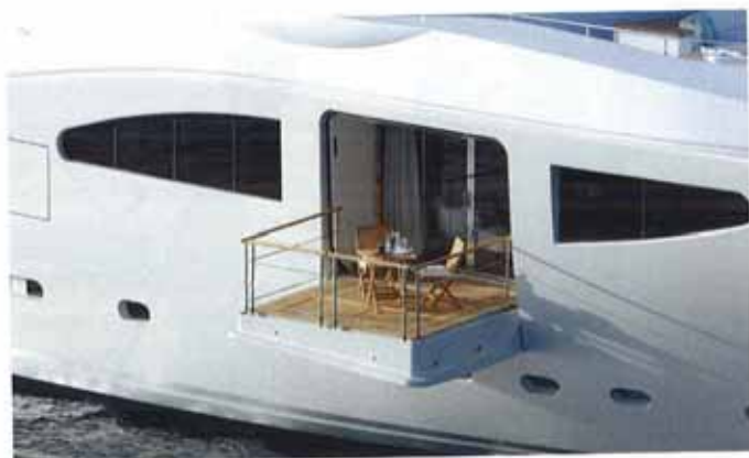
Sea Steel's handrails make a balcony safe at the flick of a switch
